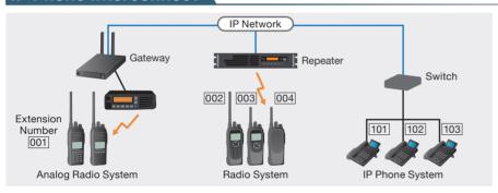
The built-in Simplified SIP server can assign extension numbers to IDAS™ radio terminals, IP advanced radio terminals, and groups of analog radio users as well as IP phones. A radio user can initiate phone calls. Phone users can make individual or group calls to connected radio users.
