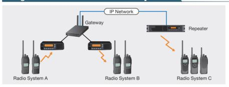
The gateway interconnects with 2 or more radio systems, even when the systems are using different bands and different categories. All received audio is bridged to opposing radio system, so a radio user can talk to all connected radio users. The built-in digital voice converter converts analog audio to IDAS<sup>TM</sup> compatible digital audio.
