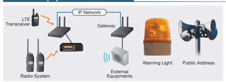
Public address system, siren, warning light and other external devices can be connected to the gateway. When detecting an emergency signal, users can start emergency notification from either a digital transceiver, IP transceiver or public address system.
