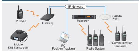
By installing a custom SIM card to the built-in LTE module, the Cotel Matrix can interconnect multiple LTE transceivers with conventional radio systems and connect IP communication terminals. GPS position information from the LTE transceivers can be received and transferred to a PC
